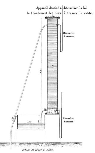
**Fig. 5** Darcy's original sand column apparatus (Darcy 1856, Plate 24, Fig.3)
