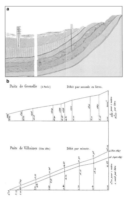
Fig. 6 Artesian well flow a Darcy's schematic of artesian flow measurements showing a geologic cross-section, and b flow rate measured as a function of the discharge elevation at two sites. A clear linear trend was observed in these and other data sets. (Darcy 1856, Plate 22)
