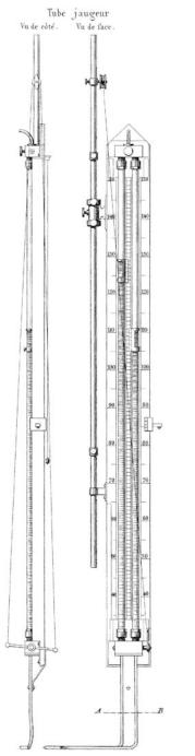
Fig. 7 The Pitot tube design used by Darcy in his 1856 report (Darcy 1856, Plate 23, Fig. 14)
